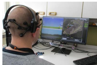
Workstation with GazePoint GP3 HD desktop oculograph and EMOTIV EEG
