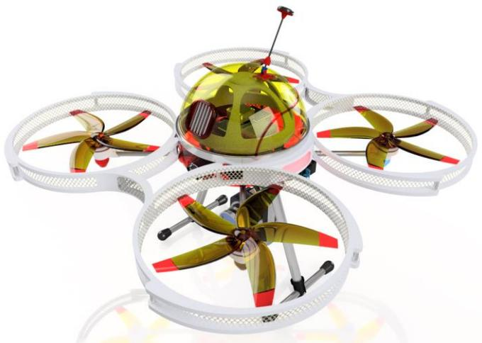
*Fig. 4. Perspective projection of the quadcopter [4]*
