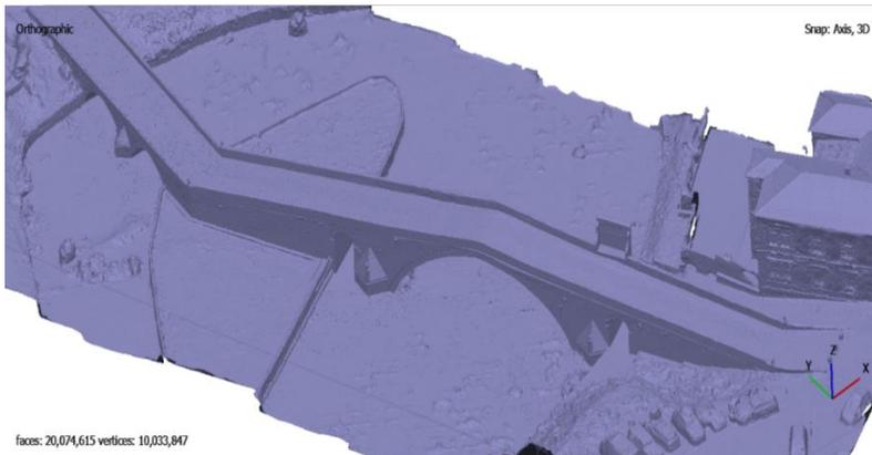
*Fig. 6. Visualisation of the polygonal model (Mesh) of the bridge*
