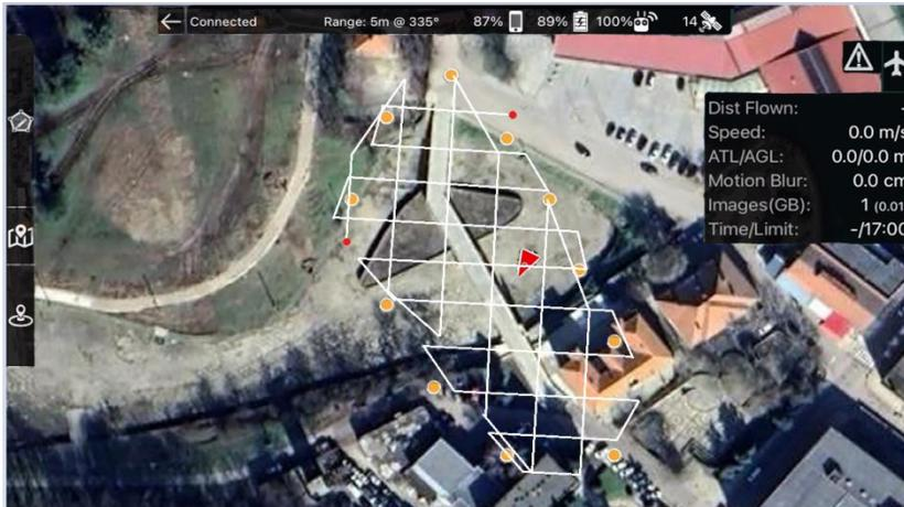
*Fig. 2. Mission plan for the "Humpback" Bridge in Harmanli, prepared through the Map Pilot Pro software*
