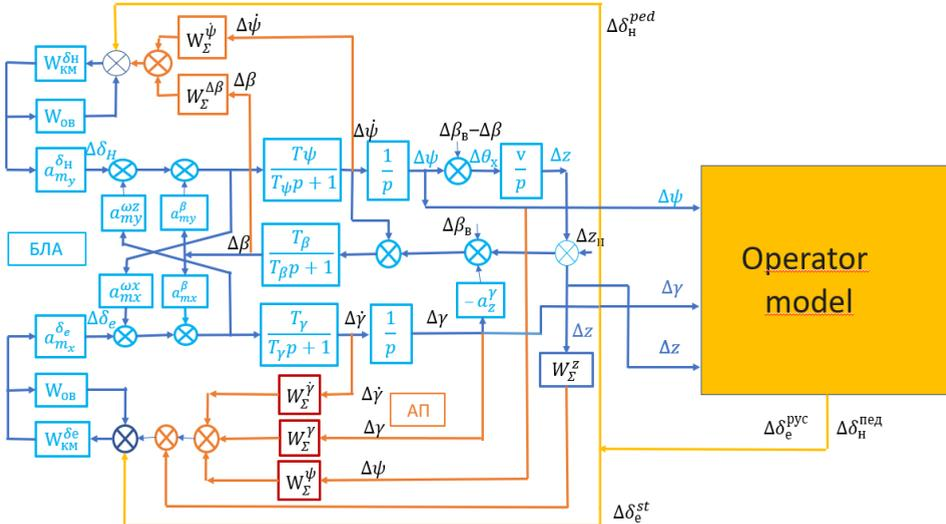
Fig. 4. Structural diagram of the "UAV-Operator" system
