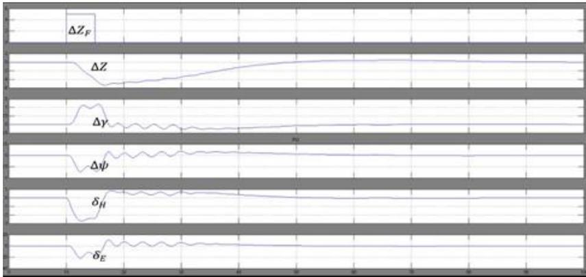
Fig. 6. Transient processes of UAV under external disturbance
