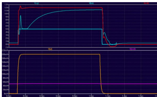
Fig. 2a. Times diagrams with “LTspise” for one driver for MOS transistor
