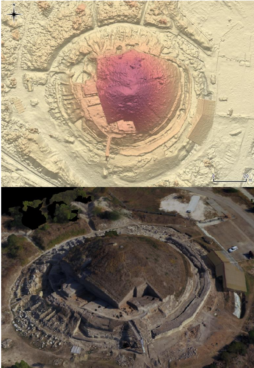
Fig. 2. Provardia-Solnitsata archaeological site. Top: DSM visualization – multidirectional hillshade with color gradient (QGIS software). Bottom: 3D texture mesh visualization (MeshLab software)
