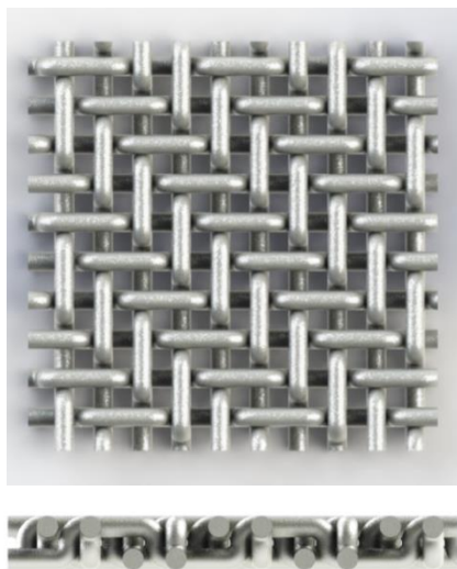
Fig. 1. Schematic representation of a twill weave of wire mesh with square cells
