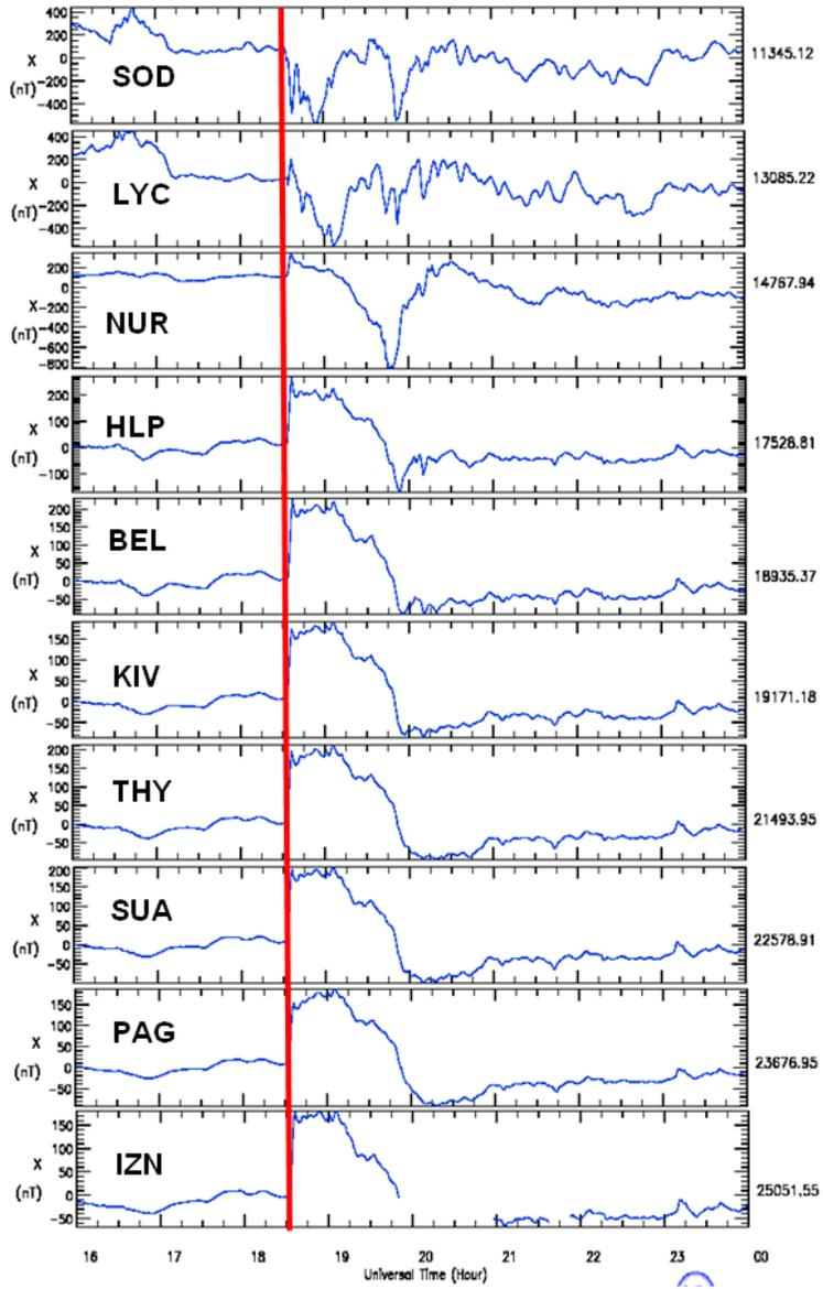
Fig. 5. X-component of the magnetic field at the selected INTERMAGNET stations during the substorm on 22 June 2015
