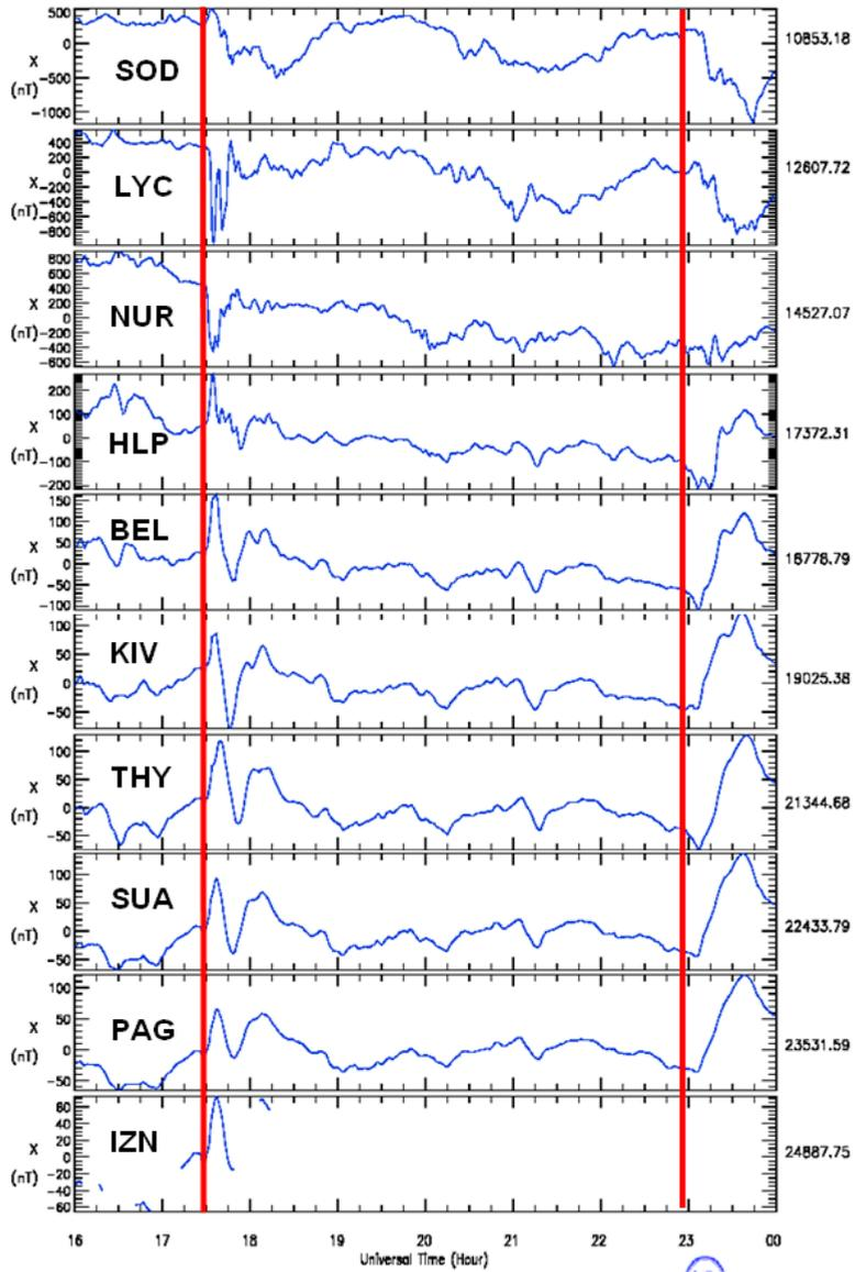
*Fig. 3. X-component of the magnetic field at the selected INTERMAGNET stations during the examined substorms on 17 March 2015*
