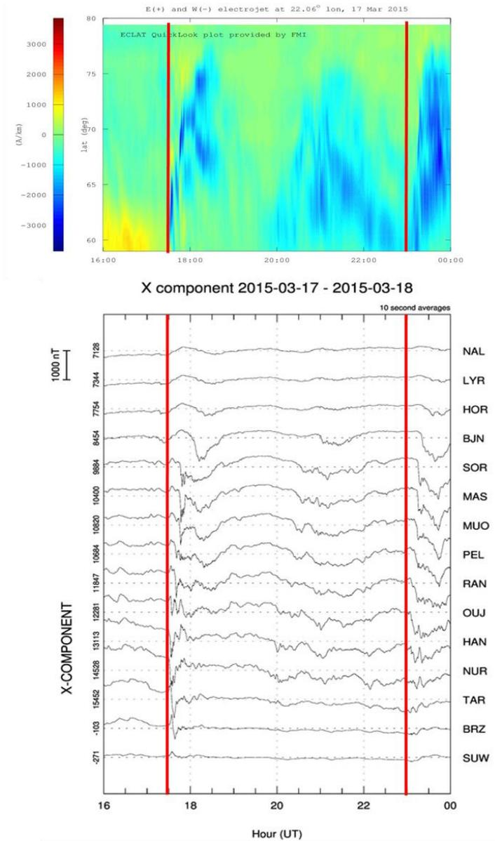
Fig. 2. Equivalent ionospheric currents (blue- negative, red -positive) – upper panel, and the X-component of the magnetic field at the IMAGE latitudinal chain SUW-NAL during the first two examined substorms on 17 March 2015 (bottom panel)
