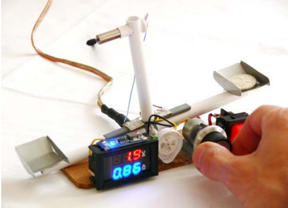
Fig. 1. Scale for measuring static thrust of micro-motors
