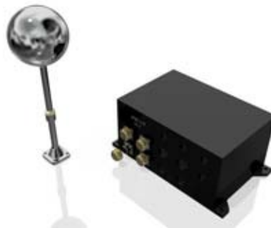
Fig. 4. Electric potential measurement equipment, project “Resonance”
