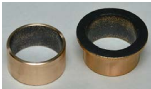
Fig. 6. Bushing without a flange (to the left) and with a flange (to the right) from the material BFG-50M [9]
