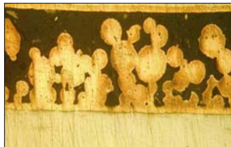
Fig. 3. Metal-fluoroplastic tape structure (Russia) [1]
