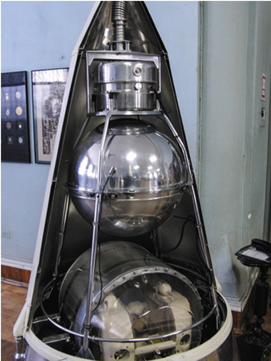
Fig. 2. Sputnik 2 was a 4-meter-tall, cone-shaped capsule designed to remain attached to the rocket that launched it into orbit on 3 November 1957. It held radio transmitters, a telemetry system, a Geiger counter, and a temperature-control system for the cabin, which carried the dog Laika. The model shown here is now at the Polytechnical Museum in Moscow.
