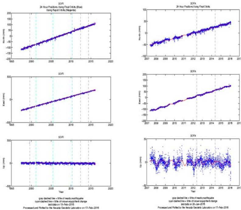
*Fig. 2. Components of the absolute velocities from the permanent stations of SOFI and SOFA, on the both sides of the Vitoshka fault*
