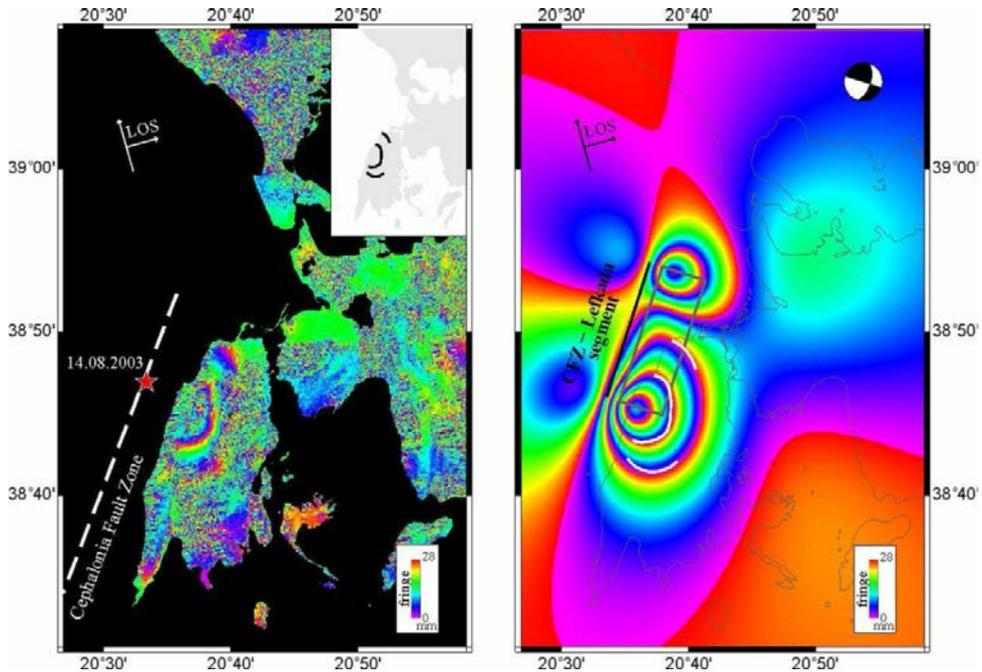
*Fig. 8. On the left – Isle Lefkada with the assessed by the method InSAR coseismic deformations and the fault activated during the shock of 2003. On the right – the model of coseismic deformations.*
