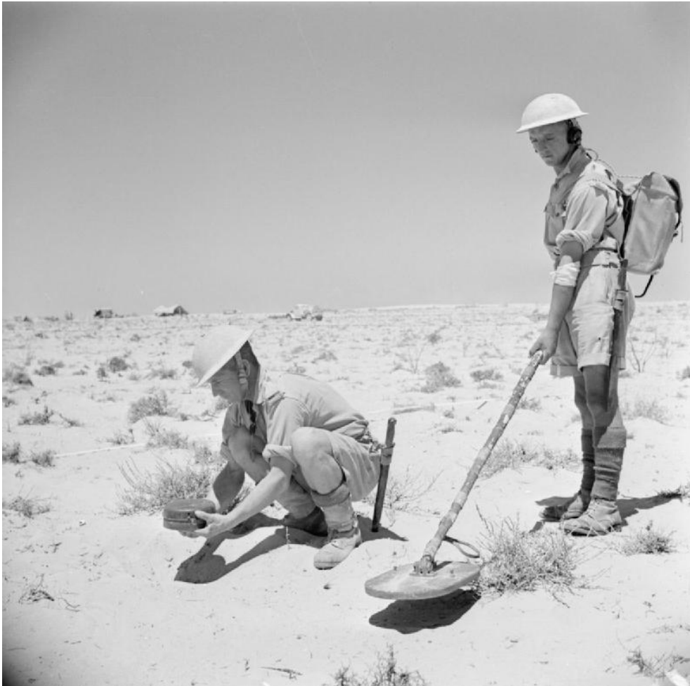
Fig. 2. Mine detector Mark I used by sappers of the Royal Engineers corps, North Africa, 28 August 1942
