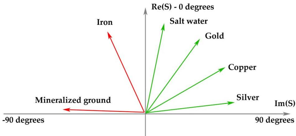
*Fig. 5. Resultant magnetic field phase shift for different metals and substances*
