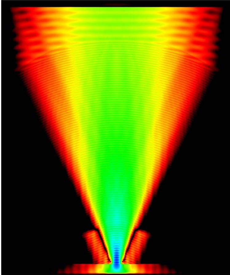
*Fig. 5. 2-D FDTD NANO-spot of about 250 nm*
