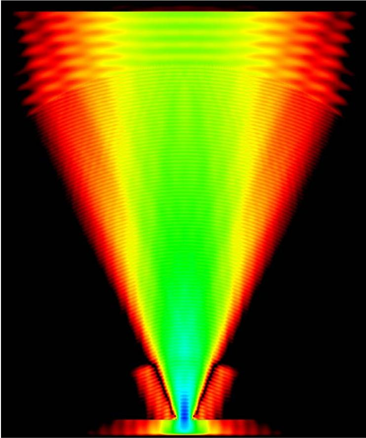
*Fig. 7. 2-D FDTD nano-spot of about 200 nm*
