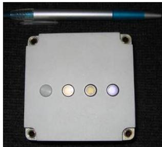
*Fig. 1. External view of R3DE instrument. R3DR instrument is with very similar external view*
