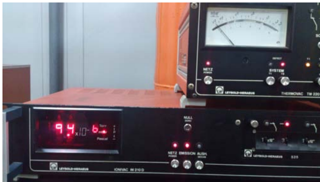
Fig. 11. Reaching the values 9,4.10^{-6} mbar of vacuum thermo chamber
