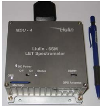
Fig. 1. LSDI with GPS receiver and SD card for continues dose monitoring at aircrafts
