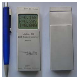
Fig. 2. LSDI with LCD display
