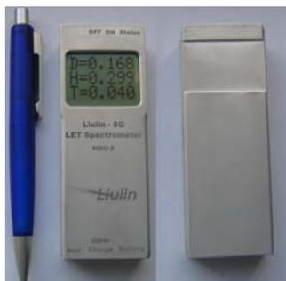
*Fig. 2. LSDI with LCD display*
