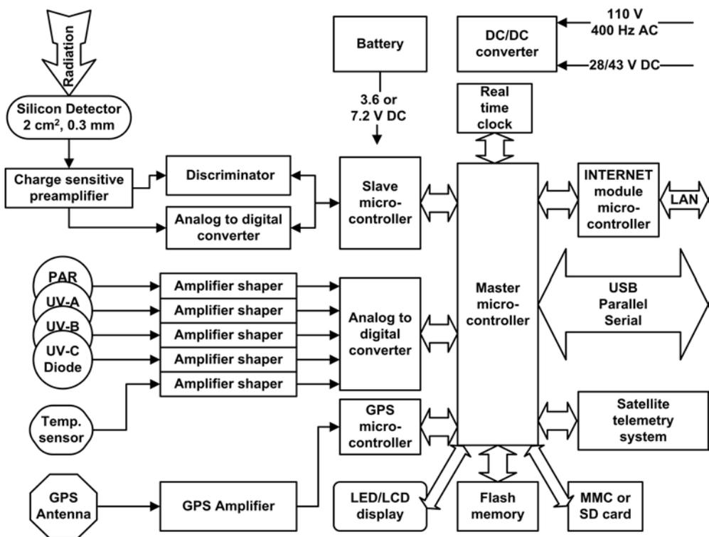
Fig. 3. Generalized block-diagram of Liulin type instruments
