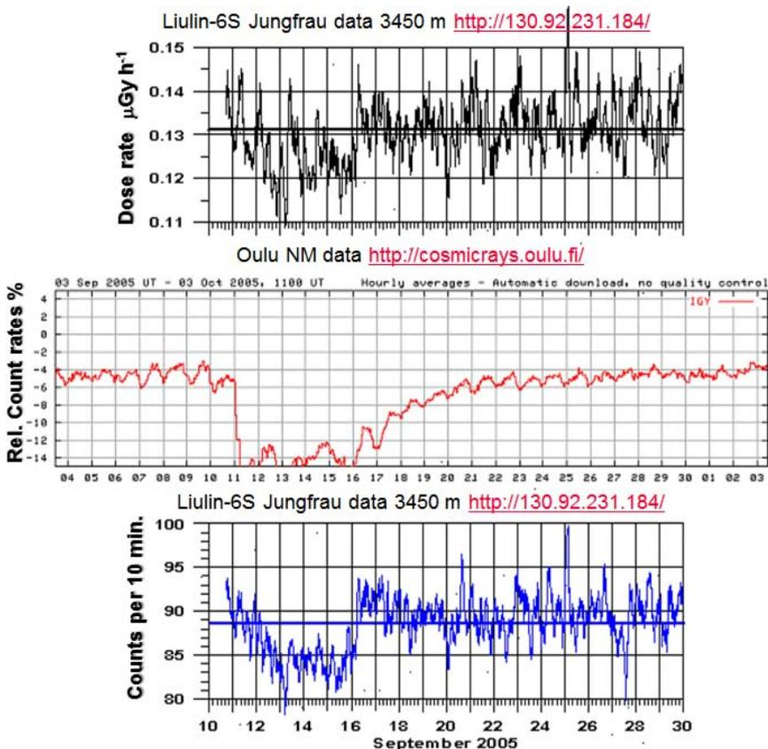
Fig. 6. Comparison of the variations of the Jungfrau dose and count rate with the Oulu NM relative count rate data around the Forbush decrease in September 2005.
