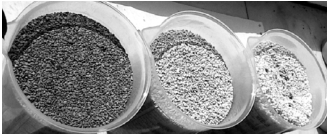
Fig. 2. A view of Turface, Balkanine, and Ekolin substrate surfaces after compaction procedures – water saturation and 50 Hz vibrations (10 min)
