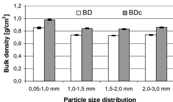
*Fig. 3. A comparative chart of the bulk densities and standard deviations for the four tested PSDs of uncompact (BD) and compact (BD<sub>c</sub>) Balkanine samples*
