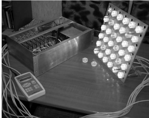
*Fig. 3. Photo of the LM-LED and the DMX Control Unit*
