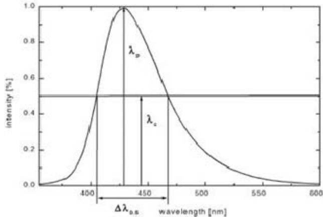
Fig. 2. Calculating FWHM (full width at half maximum)
