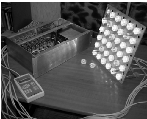
Fig. 3. Photo of the LM-LED and the DMX Control Unit
