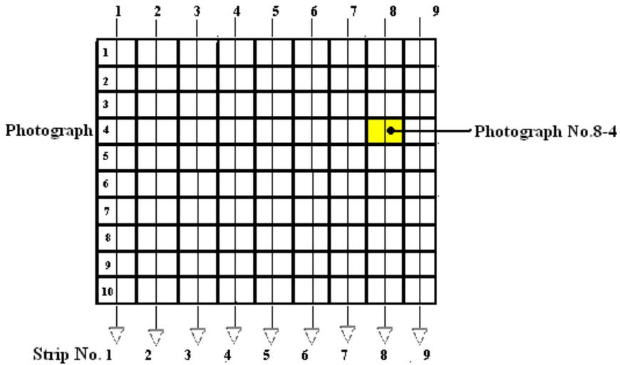
*Fig.2. Layout of strips from 1 to 9 with 10 photos in each strip*
