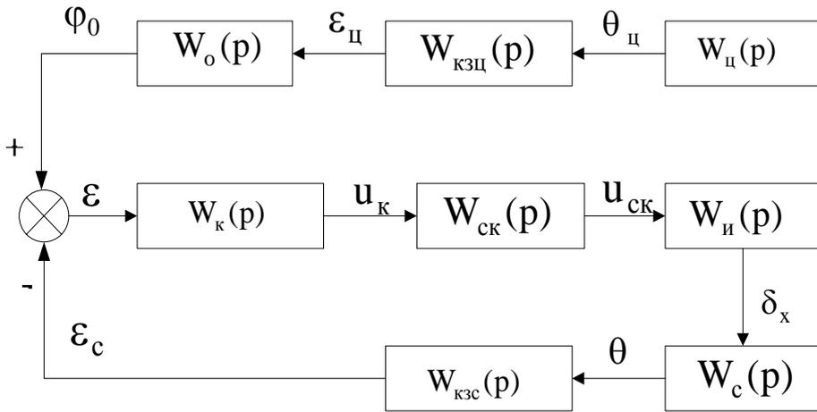
Fig. 3. Structural Diagram of ACS for UCAV
