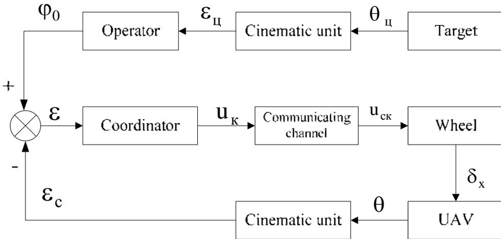
Fig. 2. Functional Diagram of ACS for UCAV
