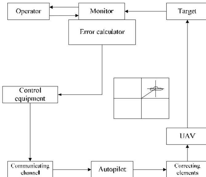
Fig. 1. Block Diagram of ACS for UCAV
