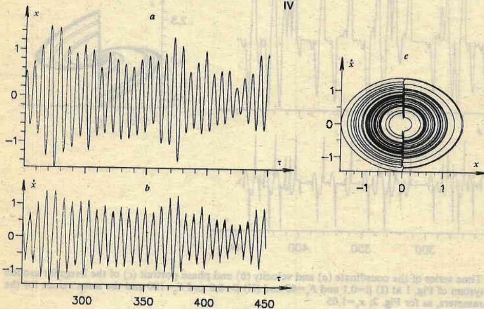
Fig. 11 gives a general idea of the nature of the pendulum oscillations for the amplitude  $A = 2.0$ , for values of  $\beta > 0.92$ , the pendulum oscillations mainly degenerate into limit or slowly damped ones.
