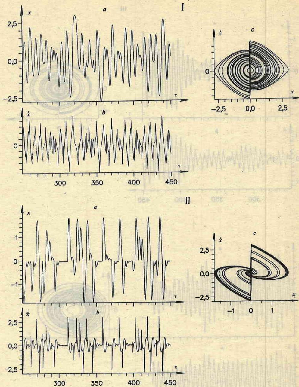
Fig. 9. Time series of the coordinate (a) and velocity (b) and phase portrait (c) of the irregular motion in the system of Fig. 1 at (I)  $\beta=0.1$  and  $F_0=40$  and (II)  $\beta=0.5$  and  $F_0=100$  and the same values for the rest parameters, as for Fig. 2;  $x_0=1.05$
