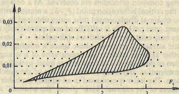
Fig. 11. Illustration on the nature of motion in the system of Fig. 1 in the plane of main parameters — damping decrement  $\beta$  vs amplitude of the external driving force  $F_0$ . The hatched area corresponds to steady-state stationary oscillations; the dots denote the area of complicated irregular pendulum oscillations
