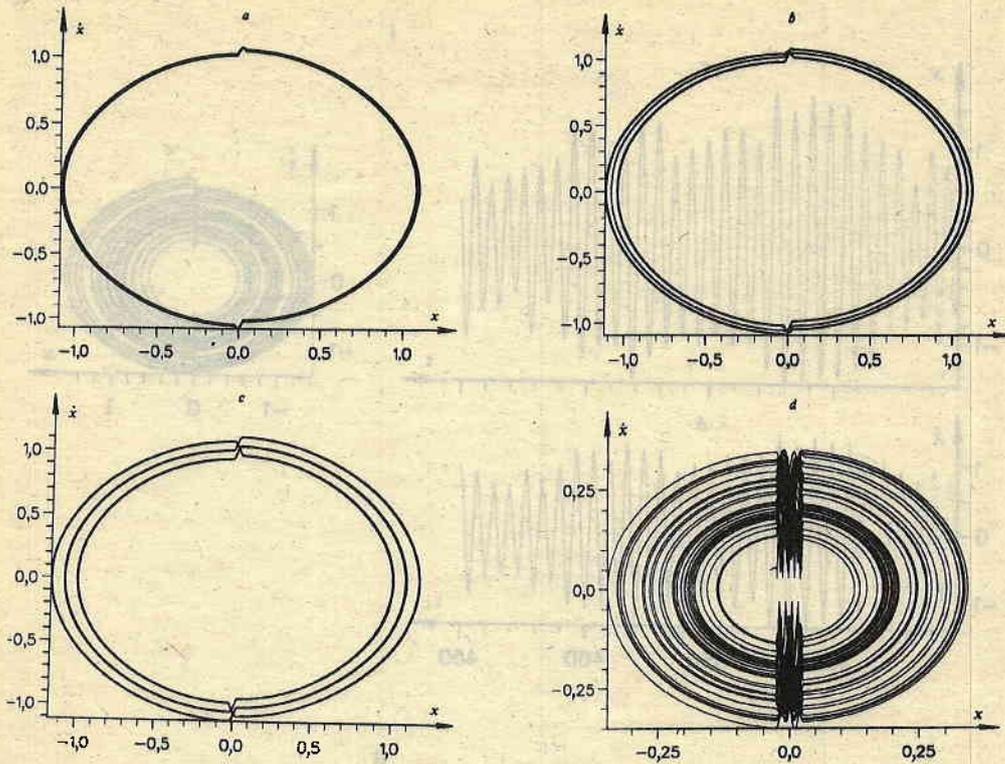
Fig. 7. Phase portraits of the motion in the system of Fig. 1 at (a)  $F_0=2,775$ , (b)  $F_0=2,8$ , (c)  $F_0=3,2595$ , (d)  $F_0=3,26$  and the same values for the rest parameters, as for Fig. 2;  $x_0=1,05$
