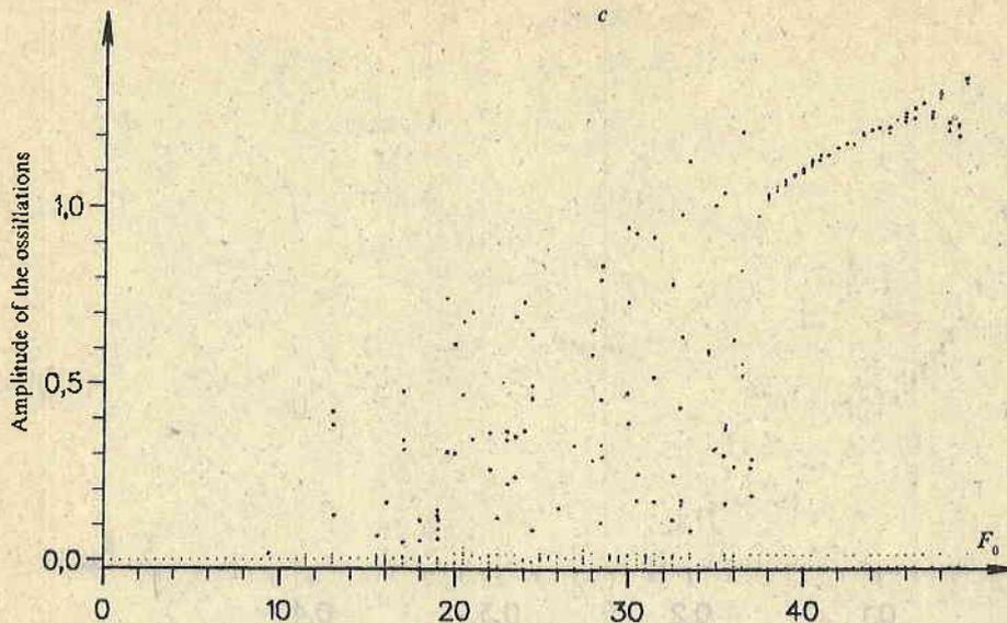
Fig. 13. Bifurcation characteristic representing the dependence of the amplitude of oscillations of a "linear" pendulum on the amplitude of the external driving high-frequency harmonic force at  $\beta=0,09$  (a),  $\beta=0,1$  (b) and  $\beta=0,225$  (c) and the following values of the rest parameters:  $x_0=0,75$  (a and b) and  $x_0=1,05$  (c),  $y_0=0$ ,  $\nu=51$ ,  $d=0,025$ ,  $F_0=\text{vary}$
