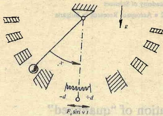
Fig. 1. Illustration of the system under consideration — a pendulum under the inhomogeneous action of an external periodic force
