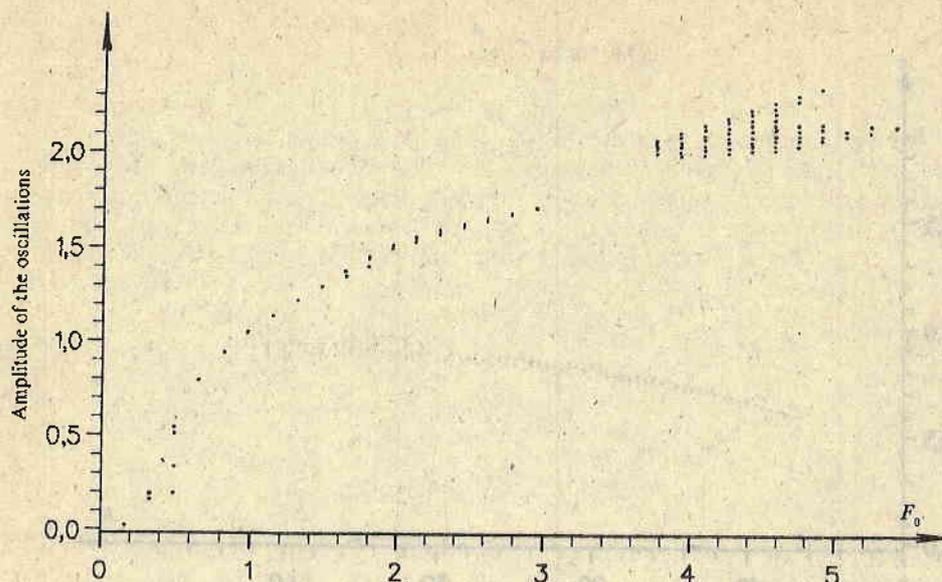
Fig. 12. Bifurcation characteristic representing the dependence of the amplitude of oscillations of a "linear" pendulum on the amplitude of the external driving high-frequency harmonic force at the following parameter values:  $x_0=1.05$ ,  $y_0=0$ ,  $\nu=51$ ,  $\beta=0.01$ ,  $d=0.025$  and  $F_0=\text{vary}$
