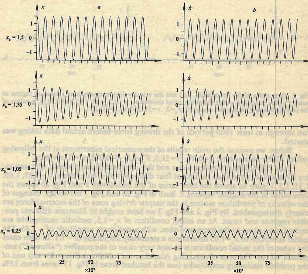
Fig. 4. Time series of the coordinate (a) and the velocity (b) at the transition process of establishing stationary motion of the pendulum at the same values of the rest parameters, as in Fig. 2
